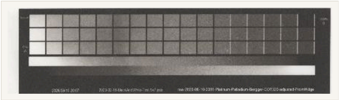
2026-08-17-0002 — a tonal step between the sixth and seventh columns, twice the banding of anything else. A coating streak, and enough to void the sheet's numbers.
